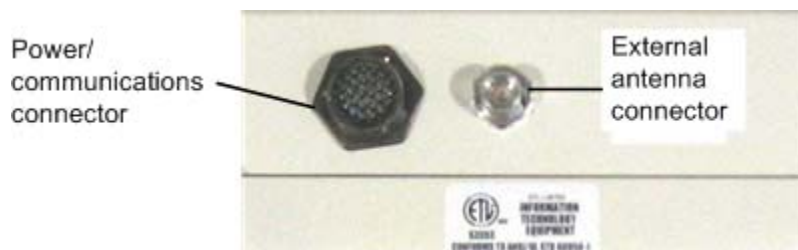
Figure 4-4 Back of Encompass 4 Reader Showing Antenna Connector
