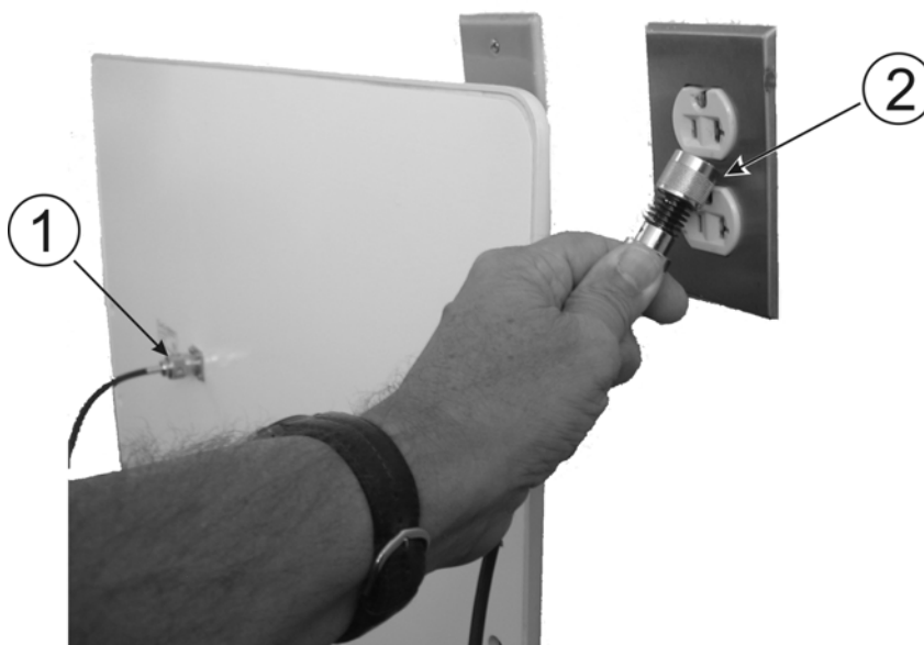
Figure 4-3 Short Load to Earth Ground
