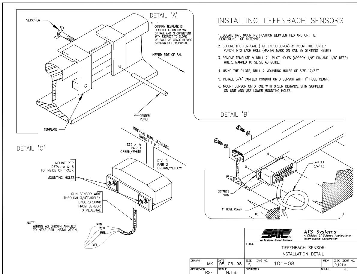
Figure 2.3: Tiefenbach transducer installation
