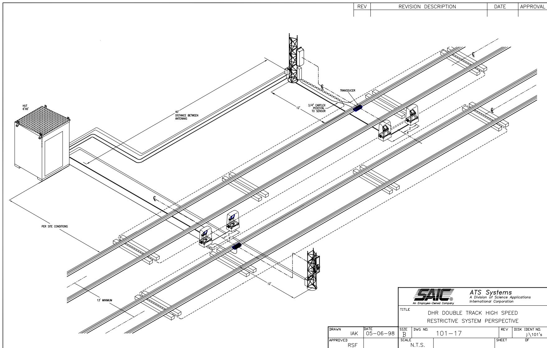
Figure C.17: DHR Double Track High Speed Restrictive System Perspective Drawing Number: 101-17
