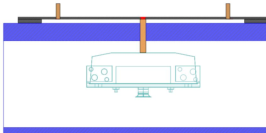
Figure 3.5: Tiefenbach transducer test plate
