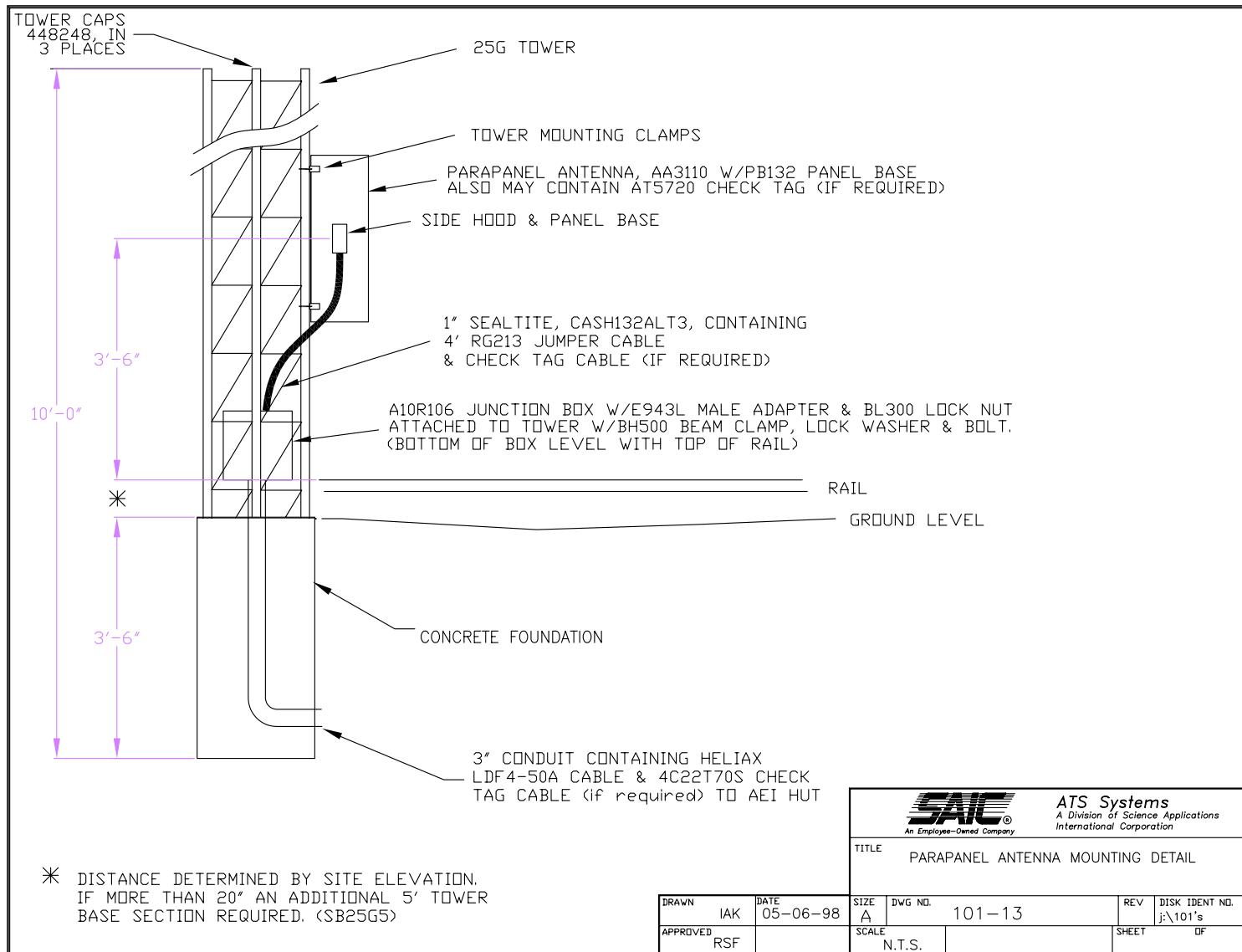
**Figure C.13: Parapanel Antenna Mounting Detail**
