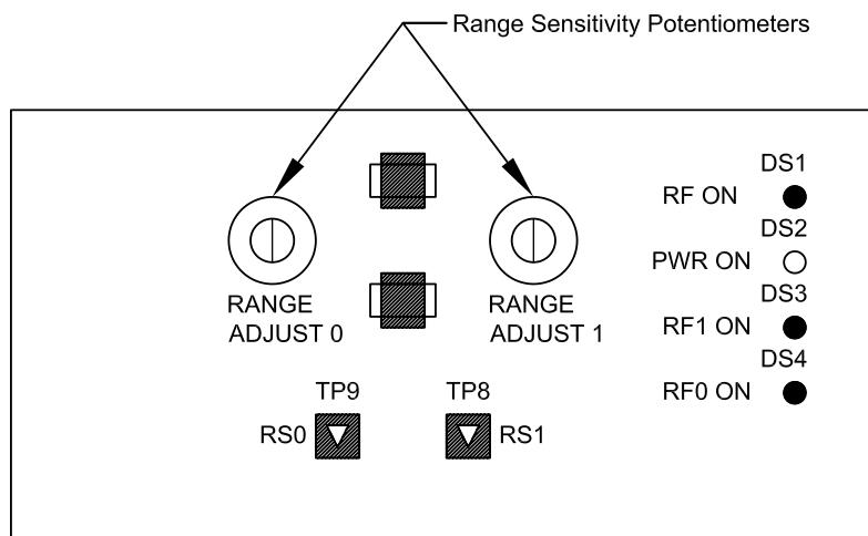
Figure 3.1: RF Module range sensitivity adjustment potentiometers
