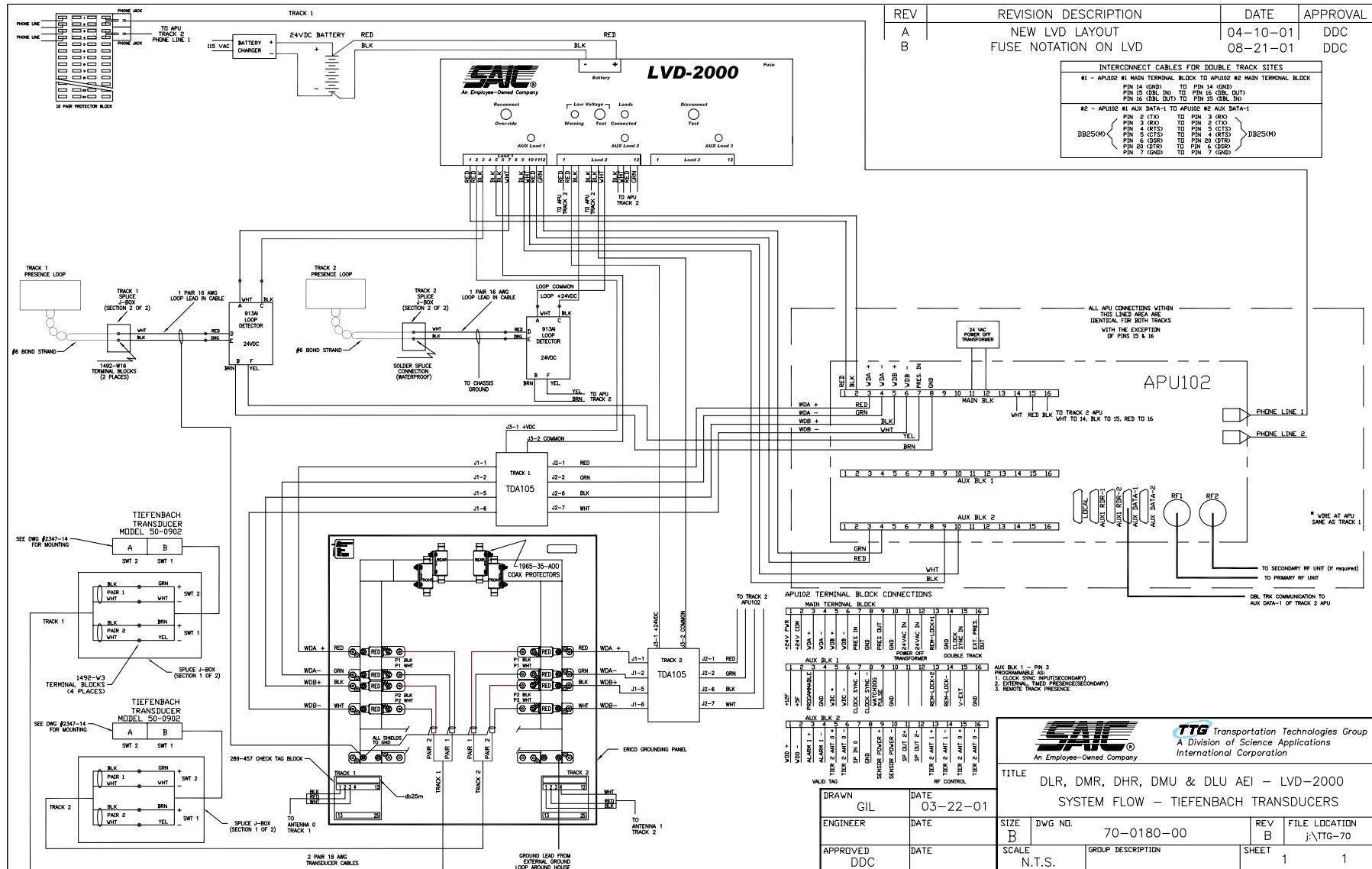
Figure C.28: DLR, DMR, DHR, DMU and DLU AEI – LVD-2000 System Flow
