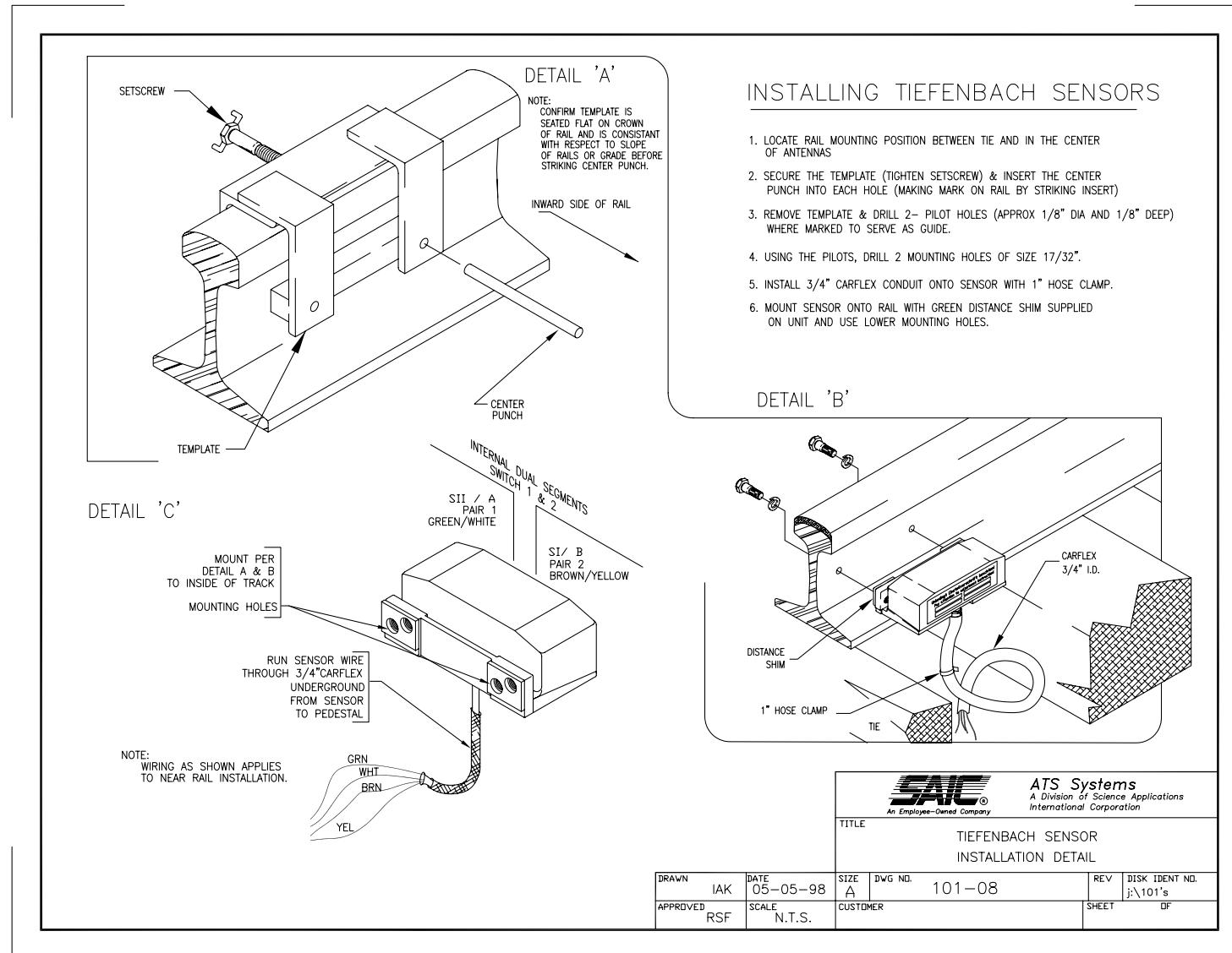
Figure C.8: Tiefenbach Sensor Installation Detail
