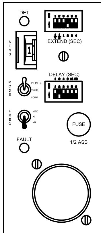
Figure C.10: Loop Detector Front Panel (913AI)
