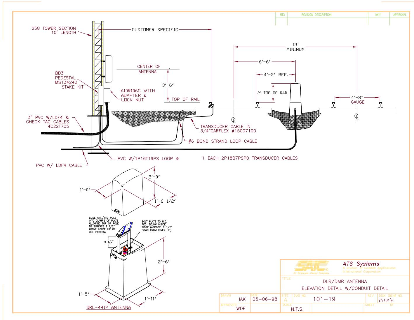
Figure C.19: DLR/DMR Antenna Elevation Detail w/Conduit Detail
