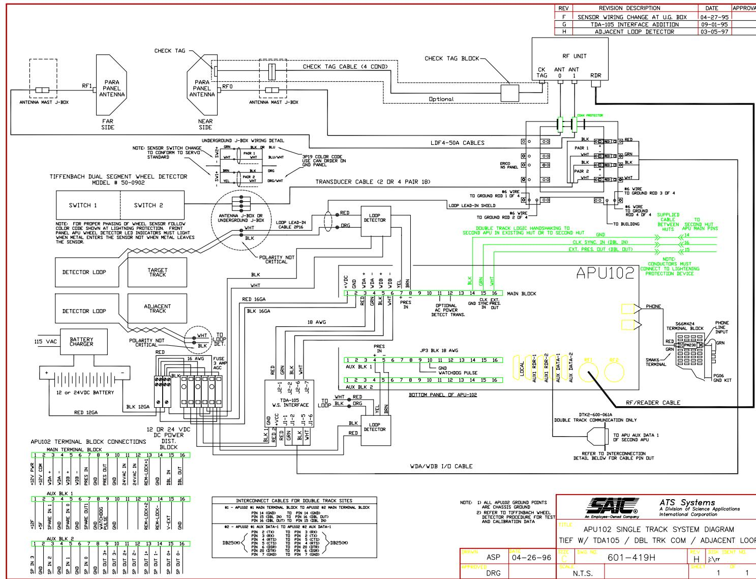
Figure C.31: APU102 Single Track System Diagram
