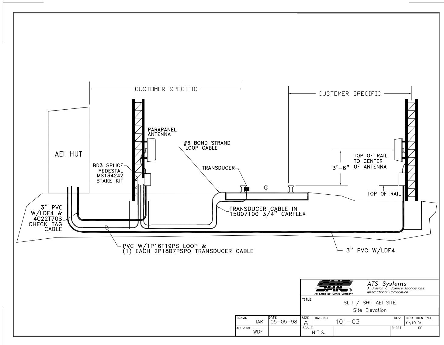
Figure C.3: SLU/SHU AEI Site Elevation
