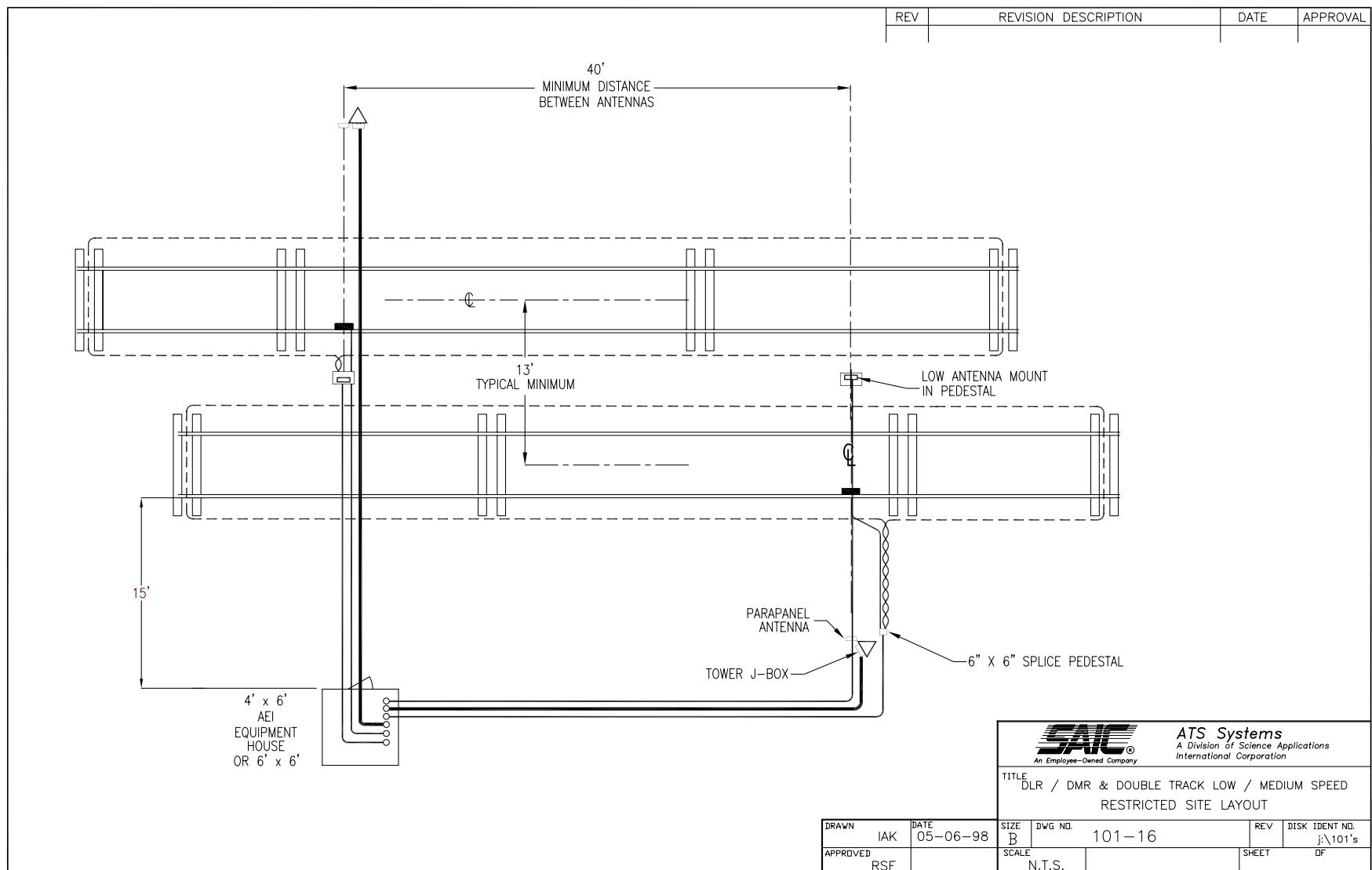
**Figure C.16: DLR/DMR & Double Track Low/Medium Speed Restricted Site Layout**
