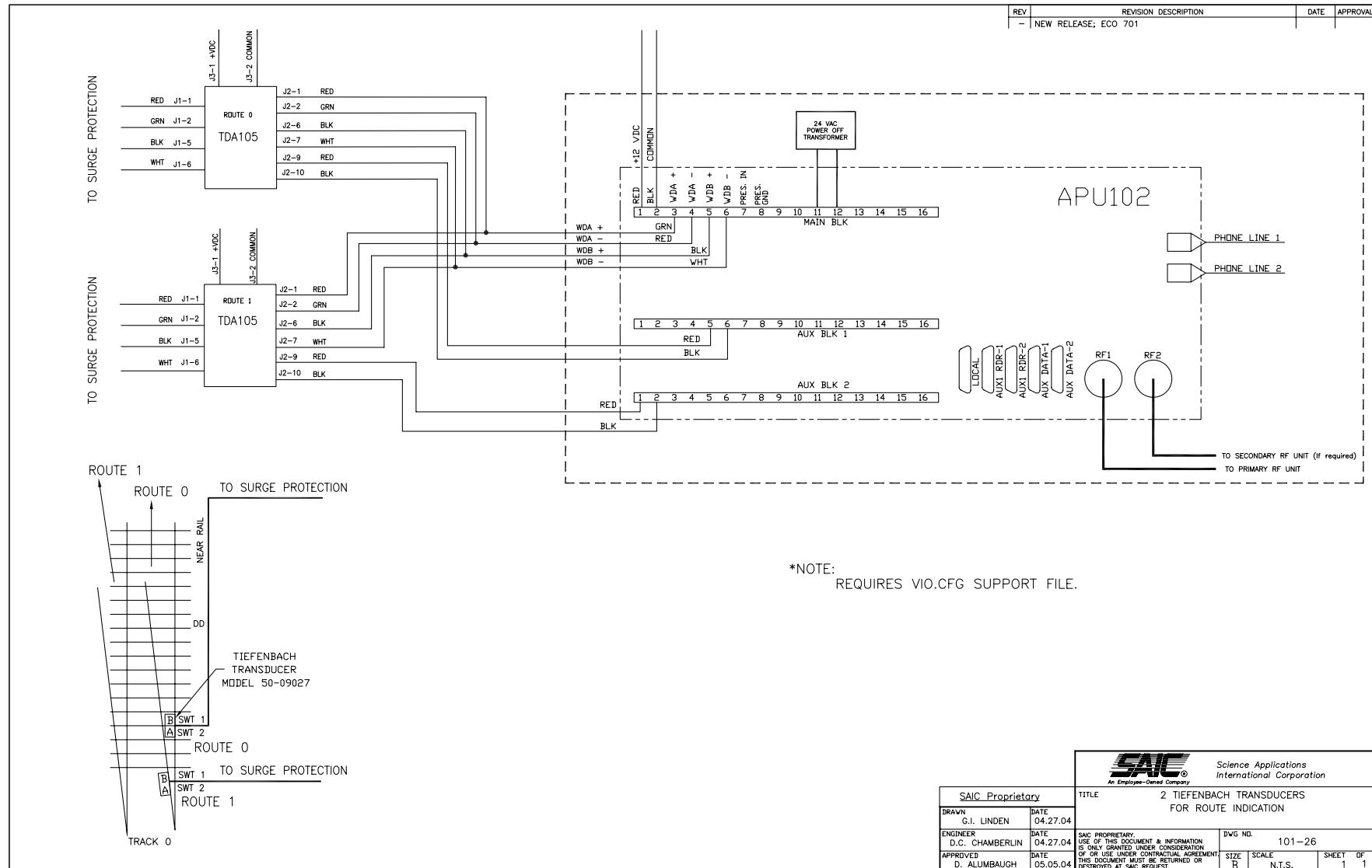
Figure C.26: SLU/SHU AEI System Flow – Tiefenbach Transducers for Route indication
