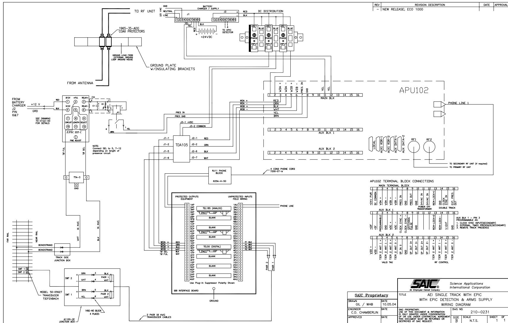
Figure C.30: SLU/SHU AEI System Flow – Tiefenbach Transducer, ARMS Power Supply, SuppressSurge Protection Panel, and Epic III Presence Circuit
