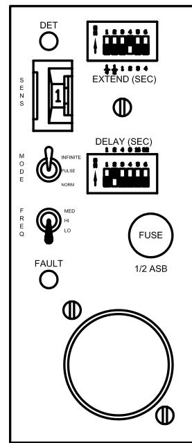
Figure 3.8: Loop detector settings
