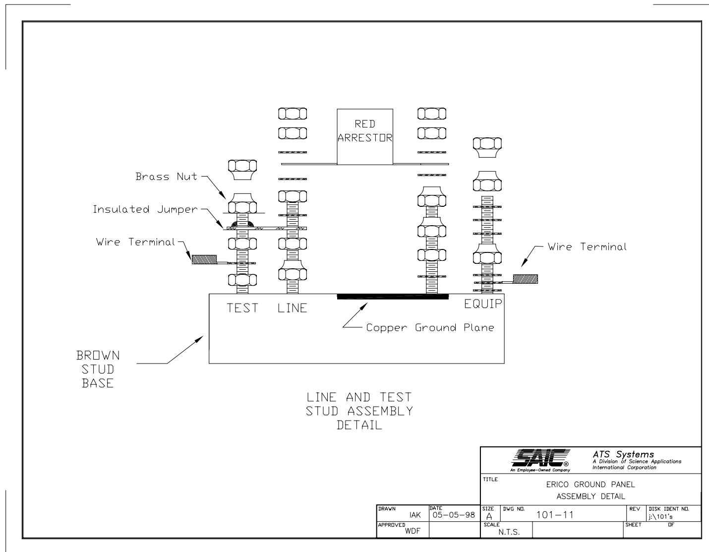
Figure C.11: Erico Ground Panel Assembly Detail
