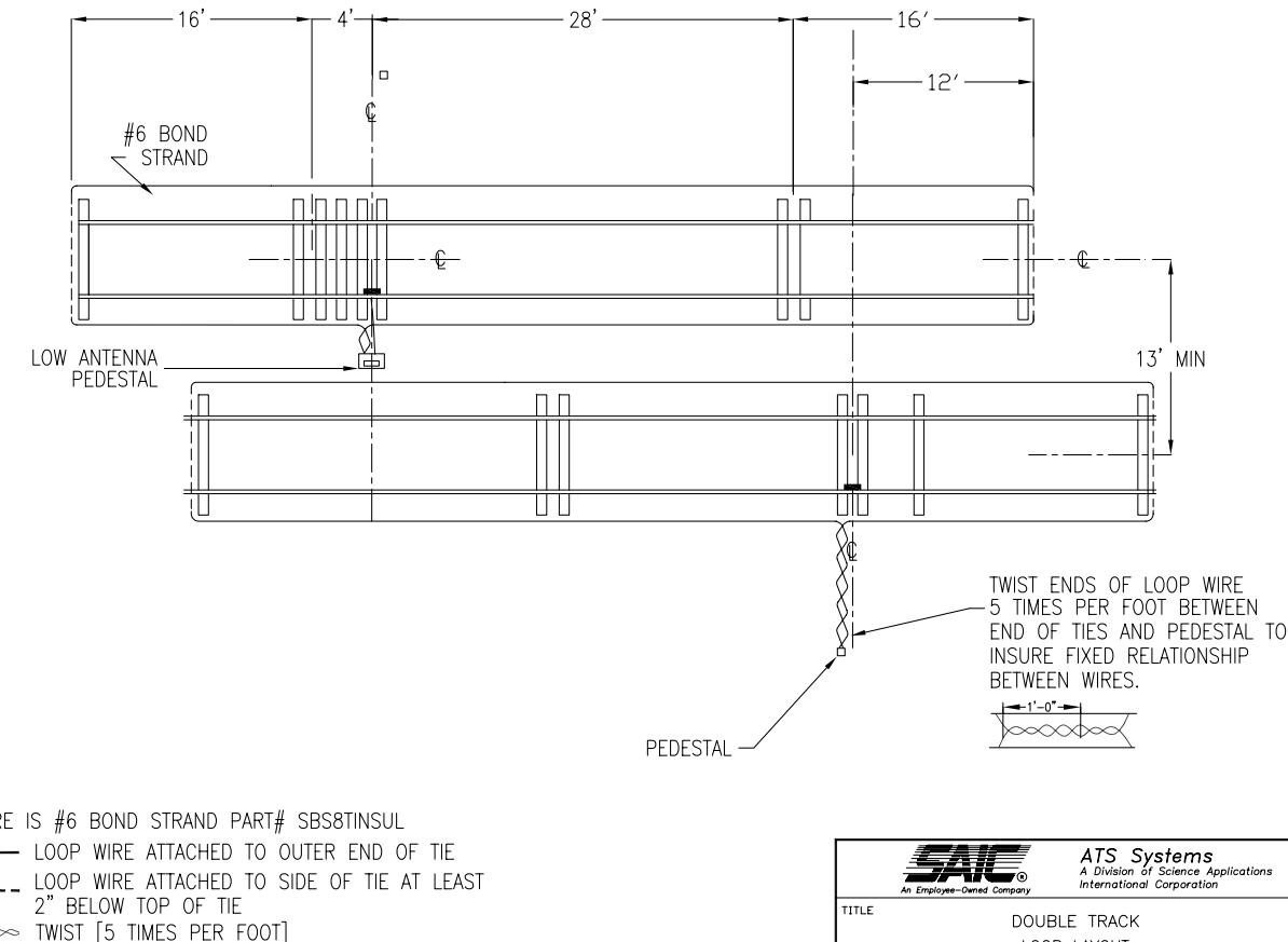
Figure C.23: Double Track Loop Layout
