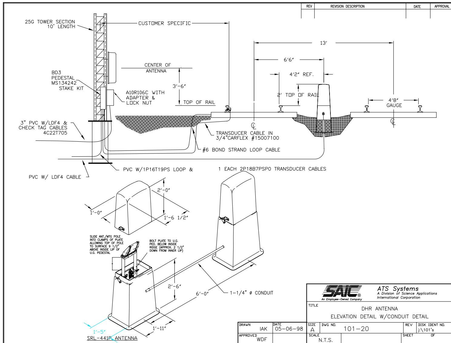
Figure C.21: DHR Antenna Elevation Detail w/ Conduit Detail
