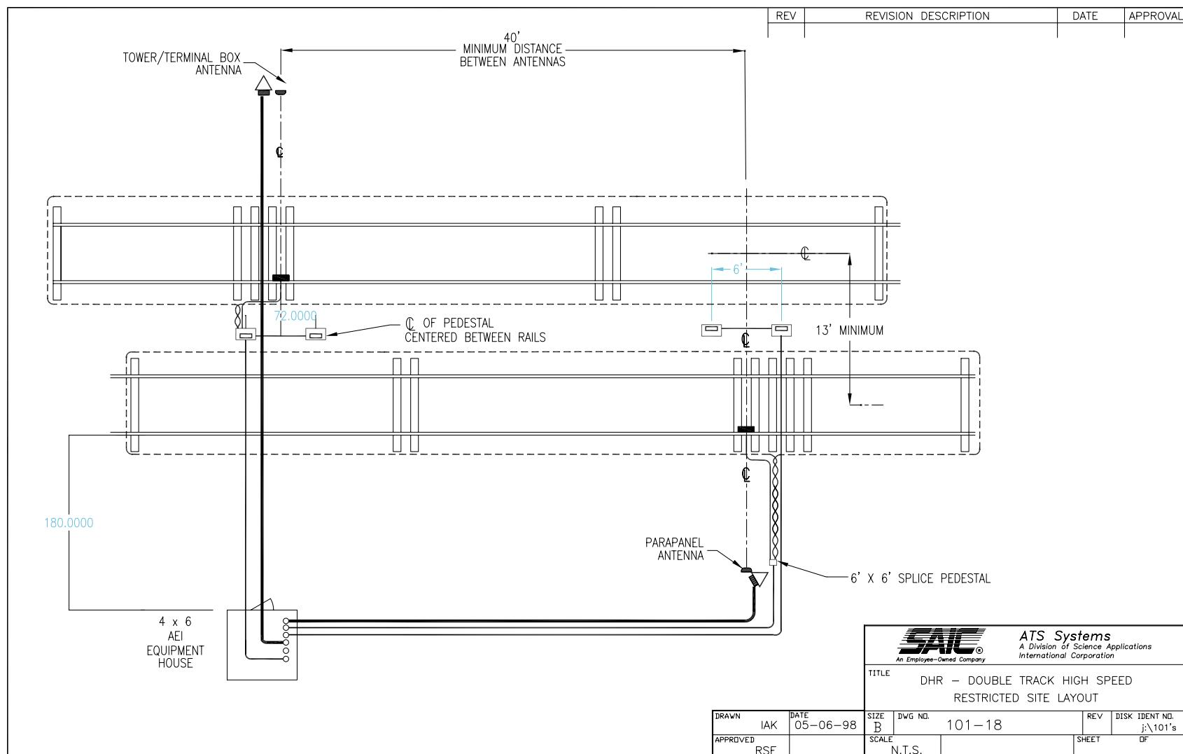
**Figure C.18: DHR Double Track High Speed Restricted Site Layout**
