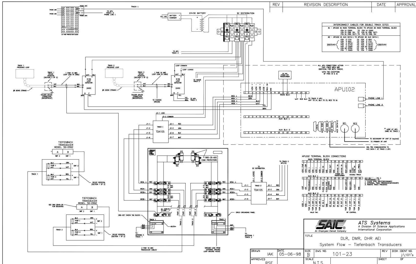
Figure C.24: DLR, DMR, DHR AEI System Flow – Tiefenbach Transducers and Presence Loop
