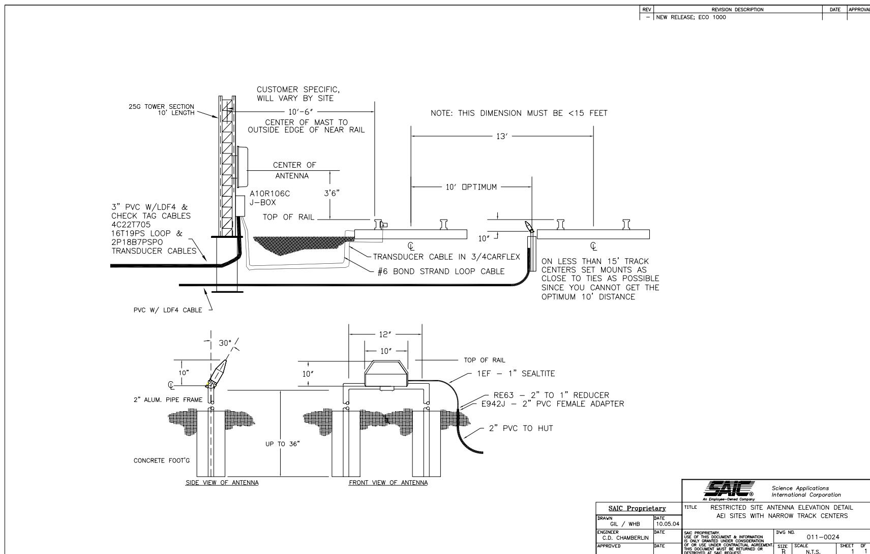
Figure C.20: DLR/DMR Antenna Elevation Detail w/Conduit Detail (Narrow Track Centers)
