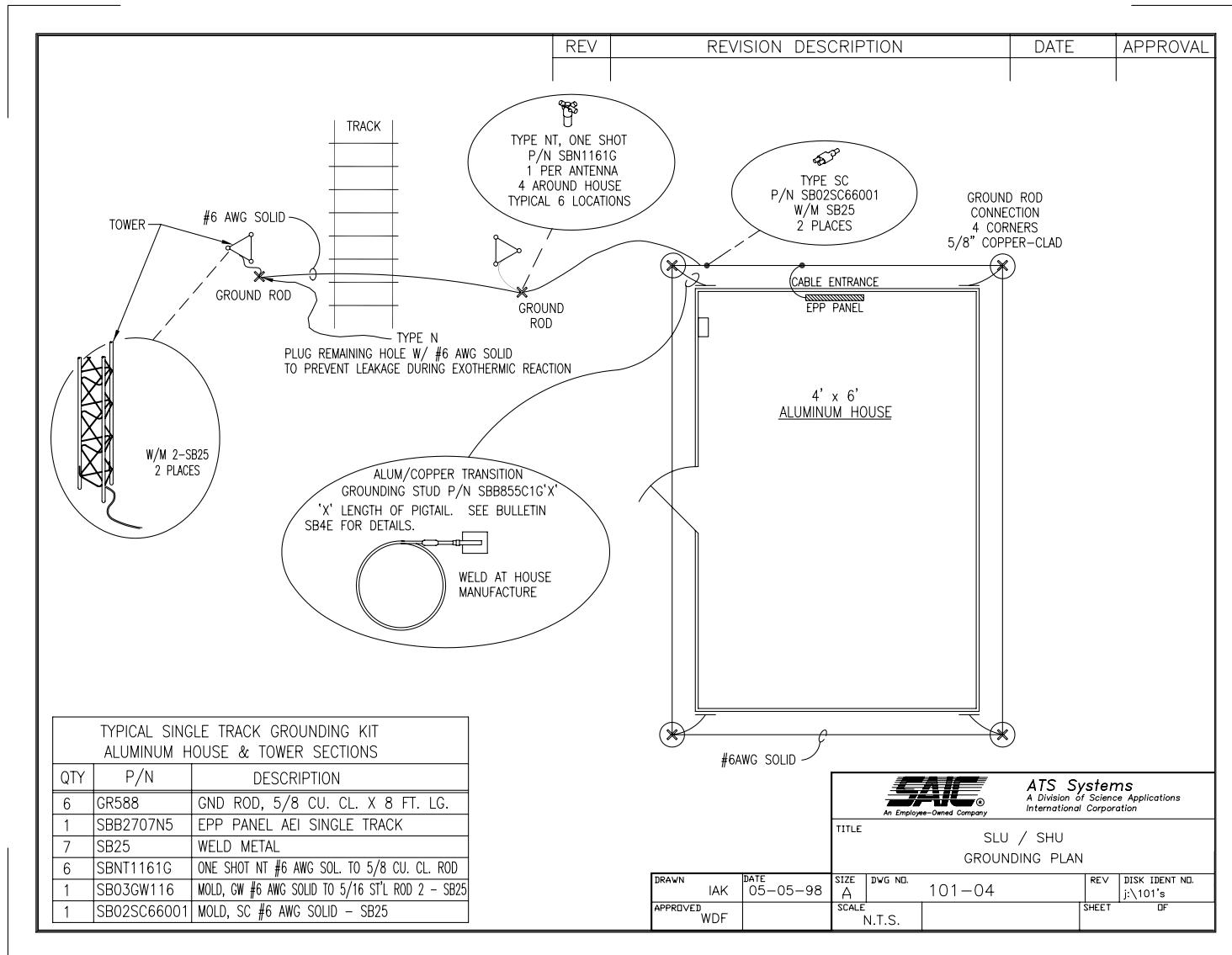
Figure C.4: SLU/SHU Grounding Plan
