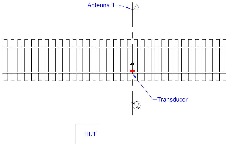
Figure 2.2: Single transducer installation location
