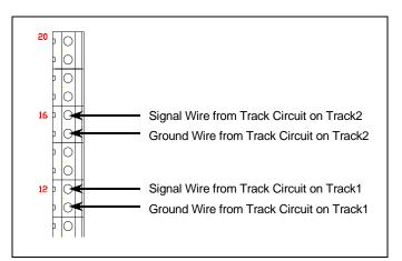
To connect the shifted-load detectors to the SmallTalk board:
