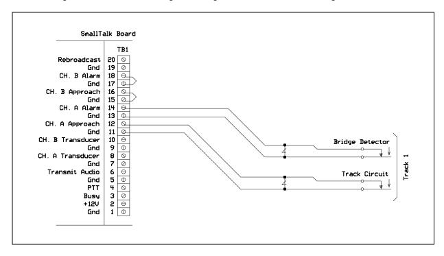
The drawing below shows the wiring for a single track with installed bridge-failure detectors.
