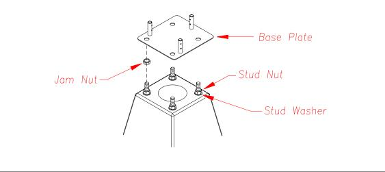
**3.** Lower the base plate onto the footer. Make the side of the base plate, with the two mounting posts, parallel to the rails. Level the base plate by adjusting the jam nuts. Remove the base plate from the footer.
