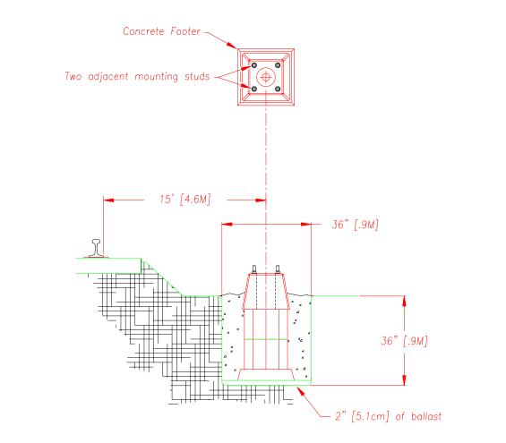
**2.** Install a 1-inch jam nut on each footer stud. Screw each jam nut until it touches the stud nut.
