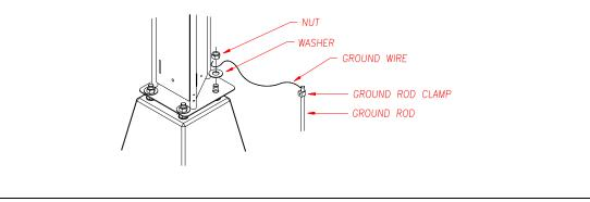
You're done installing the Solar Package. If installed correctly, the tower should be level, grounded, and attached to the footer. The solar panel should be tilted to the correct angle and facing due south.
