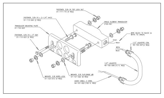
The figure below shows the parts of a transducer with the smaller mounting plate.
