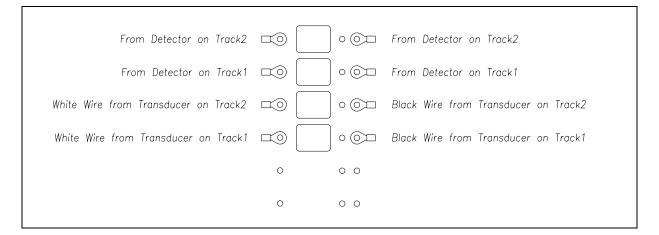
To connect the dragging-equipment detectors, bridge-failure detectors, <u>or</u> high-water detectors to the Surge Suppression panel:
