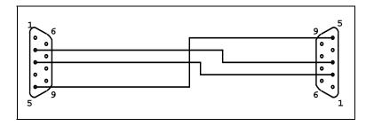
Only pins 2, 3, and 5 need to be connected for proper operation. However, a standard 9-pin-to-9-pin null-modem serial cable can be used, and one is shipped with each solar-powered SmallTalk system.
