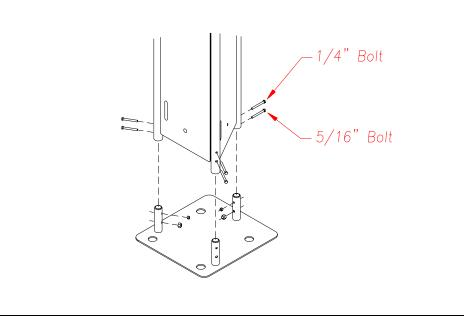
**5.** Using the supplied six bolts and nuts, secure the upper tower section to the lower tower section.
