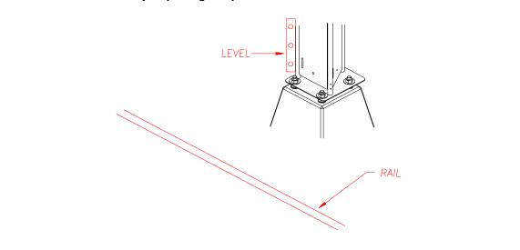
**20.** On the side of the tower, drive the 8-foot (2.4-meter) rod into the ground, attach the rod clamp to the rod, and the ground wire to the clamp. Looping the ground wire, attach it to one of the studs on the footer, between the top washer and the top nut. Tighten the nut.
