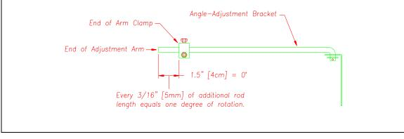
**14.** If your adjusted value is 31 through 74, 151 through 194, or 271 through 314, install the tower-mount channel and angle-adjustment bracket as shown below. Tighten the four nuts holding the two U-bolts just enough to hold the channel in place, but not too tight to keep it from moving.
