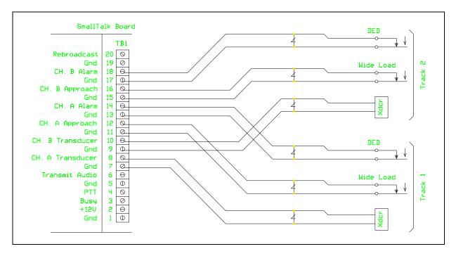
The drawing below shows the wiring for a double track with installed shifted-load detectors.
