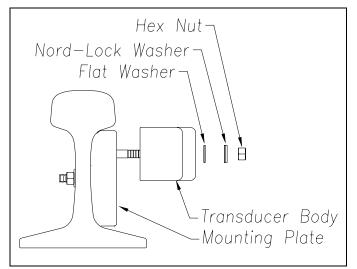
**19** By sliding it up and down, adjust the transducer body to the proper height.
