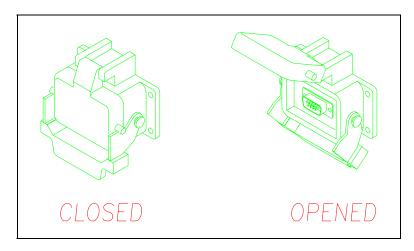
The figure below shows the serial port and its weatherproof box.
