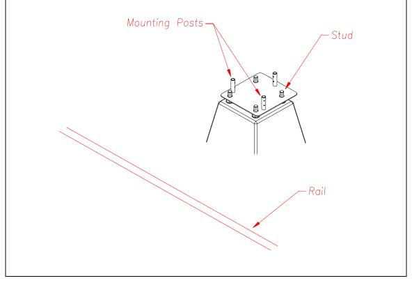
**4.** Using the supplied six bolts and nuts, secure the base plate to the lower tower section.
