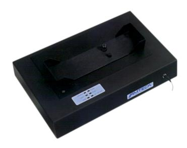
The AP4110 Programmer is used to transfer 128-bit identification codes to field-programmable Amtech<sup>®</sup> brand tags.
